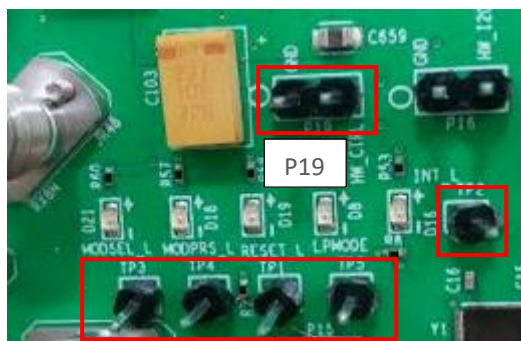
Figure 3: External Control Signals
